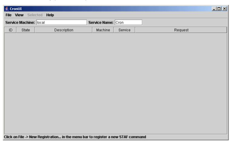
The main CronUI window displays a table of all of the currently registered STAF commands. The screen capture above shows what the table would look like if there are no registrations. The window is comprised of the following components (from to to bottom):
