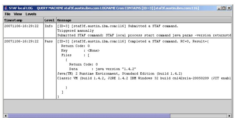
In this case, since the process returned the version immediately, the log query shows that the process has completed, and includes the information it returned.
